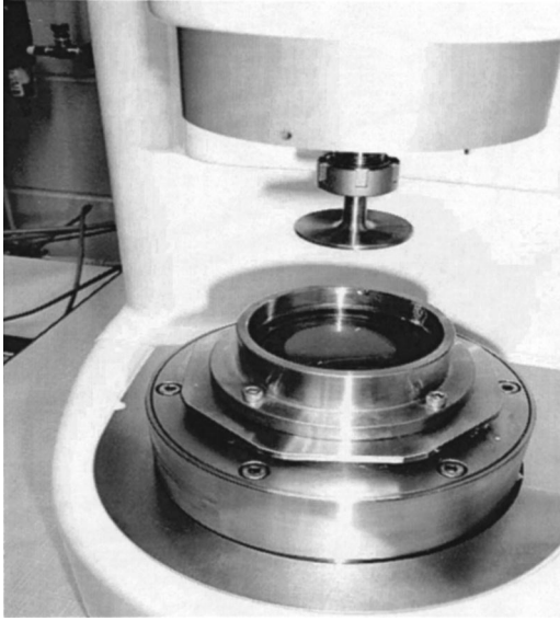
FIG. 1. Rheometer attachments for measuring the viscoelastic properties of a bio-engineered material in a cup-and-plate system filled with culture medium.
